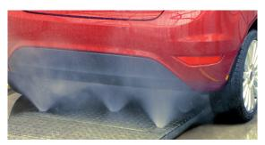
Two options are possible: static underchassis wash 10 bar [145.038 PSI], 90 L/min [19.8 gpm], and oscillating underchassis wash 15 bar [217.557 PSI], 120 L/min [26.4 gpm].
